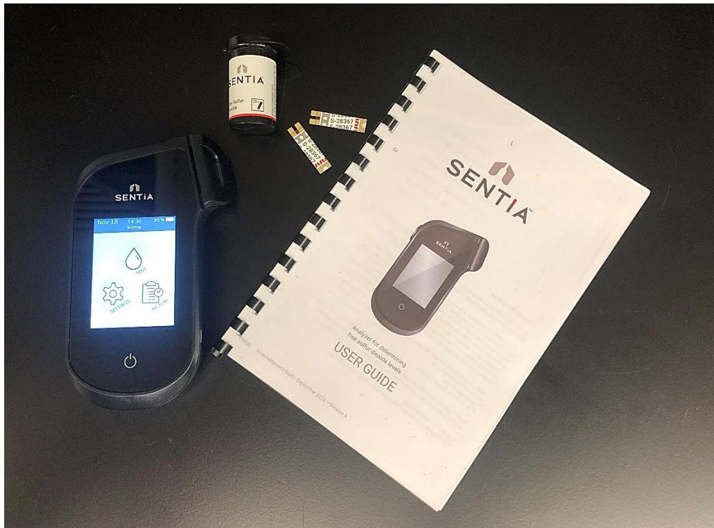
Figure 3 The Sentia™ Free SO 2 Analyzer and test strips
